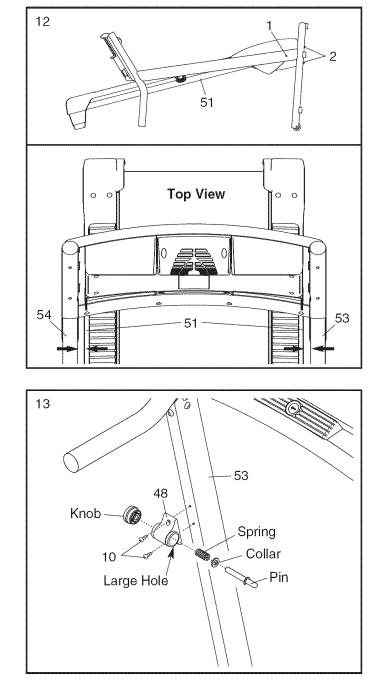
13. Attach the Latch Housing (48) to the Left Upright (53) with two M4.2 x 19mm Screws (10); start both Screws before tightening them. Make sure that the large hole in the Latch Housing is on the indicated side.
